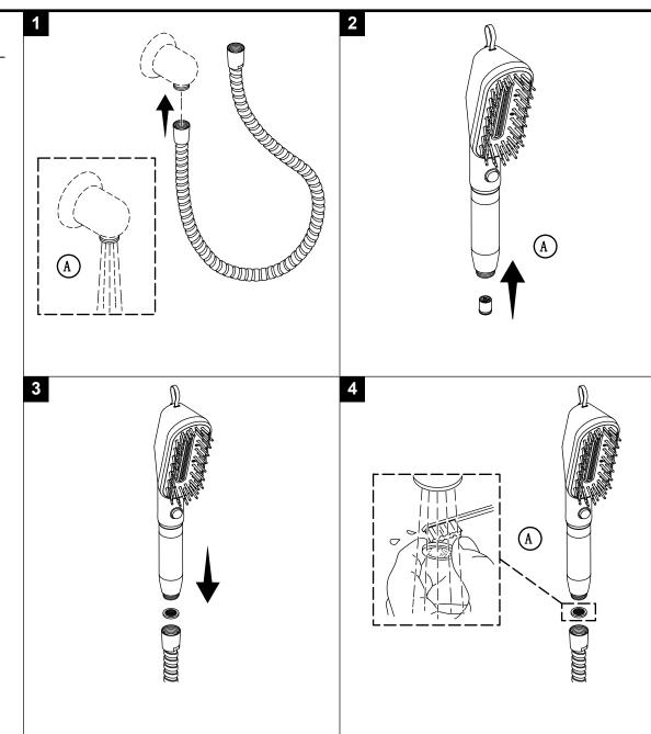
**NOTE:** The maximum operating pressure for this product is 0.5 MPa (5 bar). If the pressure exceeds 0.5 MPa (5 bar), install a pressure reducer.
