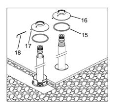
**Note:** Ensure the screws(17) is not beyond internal surface of escutcheons(16) before installation. Or adjust them by hex wrench(18). In order to avoid damage the riser tube surface.
