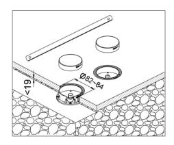
1. When the distance between top surface of bases(2) and bottom surface of tiles is ≥19mm(bottom surface of tiles is above the MIN line on the protector), and the distance between top surface of base and that of tile is≤34mm(top surface of tiles is under the MAX line on the protector):
