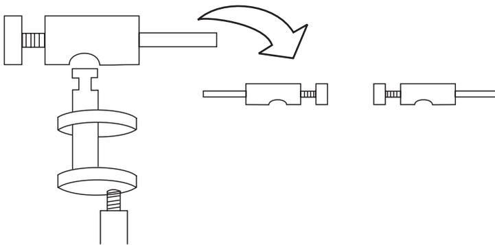
1. Insert the hinge into the mounting hole, put on the dilatant and nut, then tighten the screw on the hinge by screwdriver slightly (for another installation, dilatant is not supplied).
