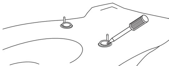
5. Insert toilet seat, Put on the flange fit it by bolt and screw.
