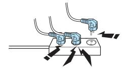
Do not pull the power cord to disconnect the machine, only holding the wire, or touch the power plug with wet hands.
