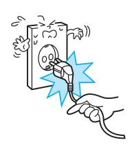
Push the power plug fully into the socket outlet.
