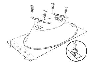
2). Using a level, adjust the height of the feet by loosening the lock nut (1) and turning the feet as shown (2) below.
