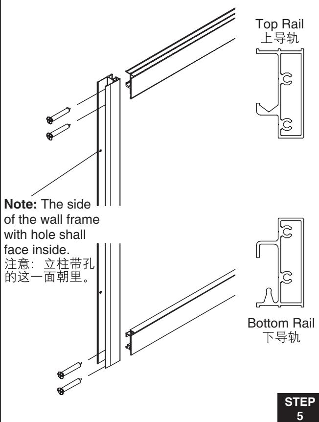
Fix the left and right frames by the bracket blocks.
