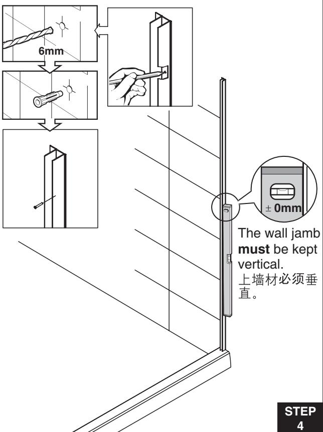
Fix the top and bottom rails to the side wall frame.
