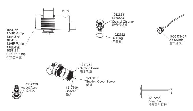
Refer to roughing-in for service parts page of bath with electronic drain. 配电子排水浴缸的维修零件图参见尺寸图。
