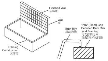
5). Sunken Installation: Refer to rough-in notes on page 1 to 6 for cut-out details. Make sure the whirlpool is supported by the supporting feet on the bottom of the whirlpool.
